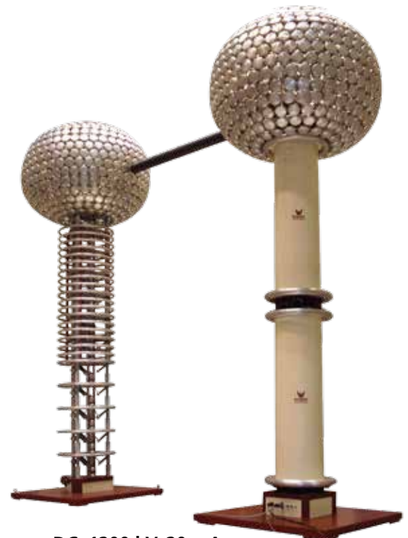
DC, 1200 kV, 20 mA
