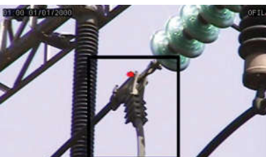
In transmission Corona on recloser
