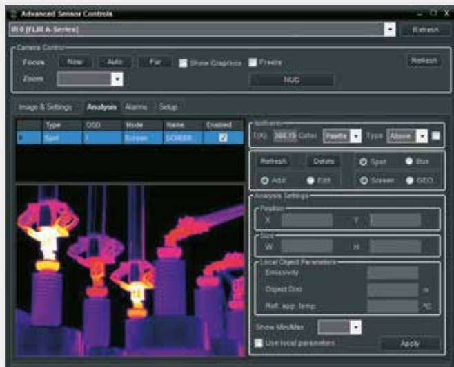
With FLIR Sensors Manager you can geo-reference your thermal imaging camera and easily change image settings, alarm conditions,...
