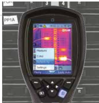
FLIR i3, temperature in 3,600 spots
