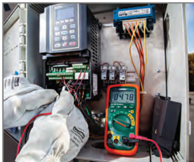
Low Pass Filter (LPF) ensures accurate AC Voltage measurements on a variable frequency drive.
